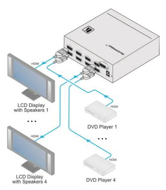
Figure 3: Connecting the VA-4H 4-Channel HDMI EDID Controller
